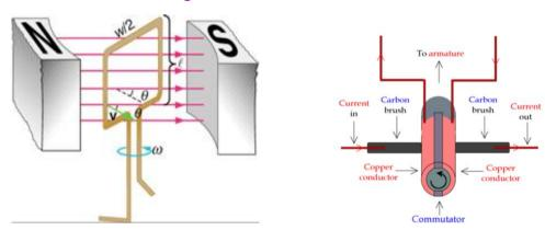
A DC Motor requires a split-ring <u>Computator</u> to function. The split-ring commutator allows for a <u>Change</u> in the direction of the <u>Current</u> in the coil. If you didn't change the direction of the current in the coil, the coil would only turn until it found an equilibrium position. The geometry of the commutator makes certain that it keeps <u>Changue</u>.
